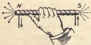
FIG. 328. — Rule for Determining the Poles of a Helix Carrying a Current.
